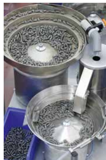
Unit that divides and doses miniature screw springs
