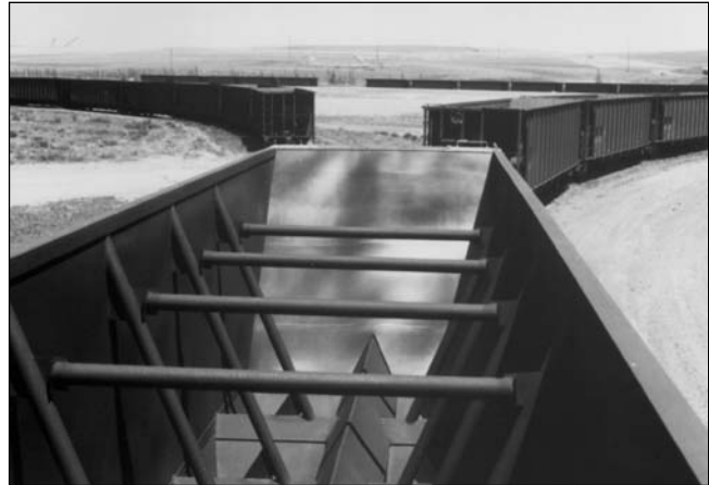
Basin Electric railcars with TIVAR® 88-2 liners installed.
