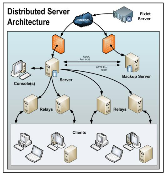
In the case of a failover, the Relays will automatically find the backup server and reconnect the network.
