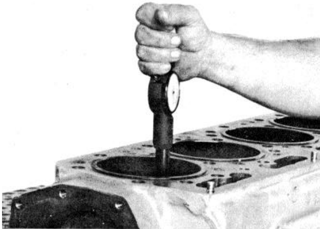
Fig. 14-12. Measure The Bore Of The Liner.
