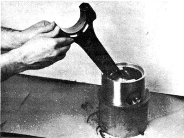
Fig. 14-15 (N114248). Install The Upper Bearing Shell Into The Connecting Rod.
