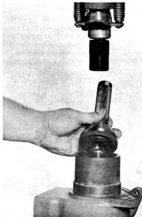
Fig. 8-29 (N10872). Install The Seal Into The Housing
