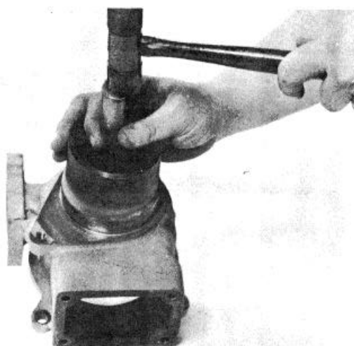
Fig. 8-17 (N10860). Remove The Oil Seal From The Housing.
