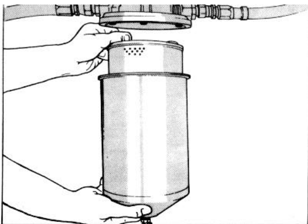
Fig. 2-20, (OM1021L). Installing replaceable fuel filter element
