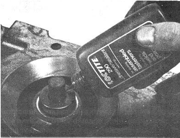
Fig. 8-52 (UW102). Apply Loctite Between The Shaft And The Cup Seat.
