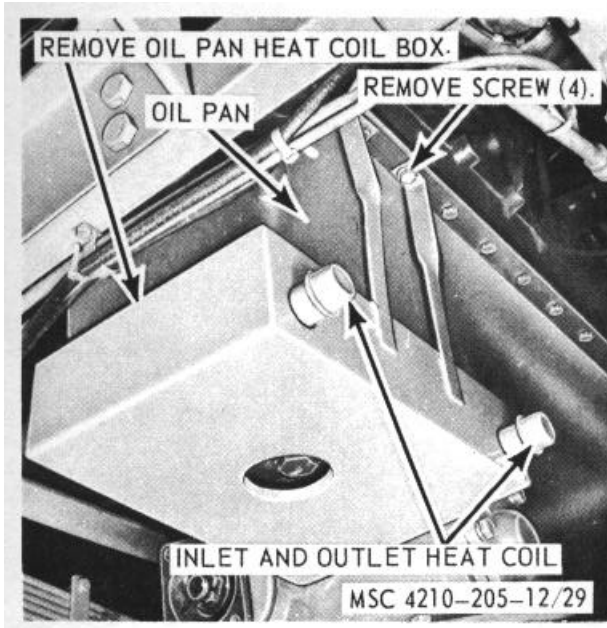
Figure 29. Oil pan heater adapter, removal and installation.
