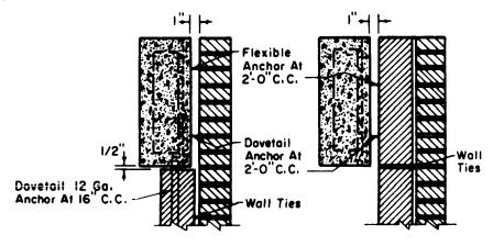
WALL ANCHORAGE TO CONCRETE BEAM
