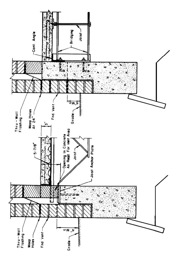
Fig C-8. Typical cast-in-place or precast concrete grade beam with steel bar joist floor framing.
