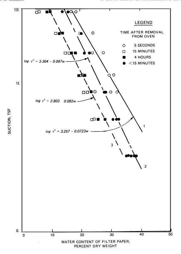
Figure B-3. Calibration of filter paper.
