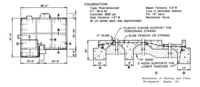
Figure 6-6. Post-tensioned slab in Lubbock, Texas, for single-family, single-story, minimally loaded frame residence.
