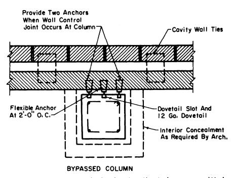
Note: Ties to column are required only when ties to beam are omitted.
