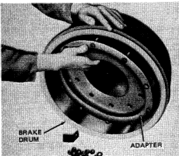
LOOSENING ADAPTER FROM BRAKE DRUM
