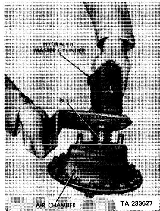
SEPARATING OR INSTALLING AIR CHAMBER
