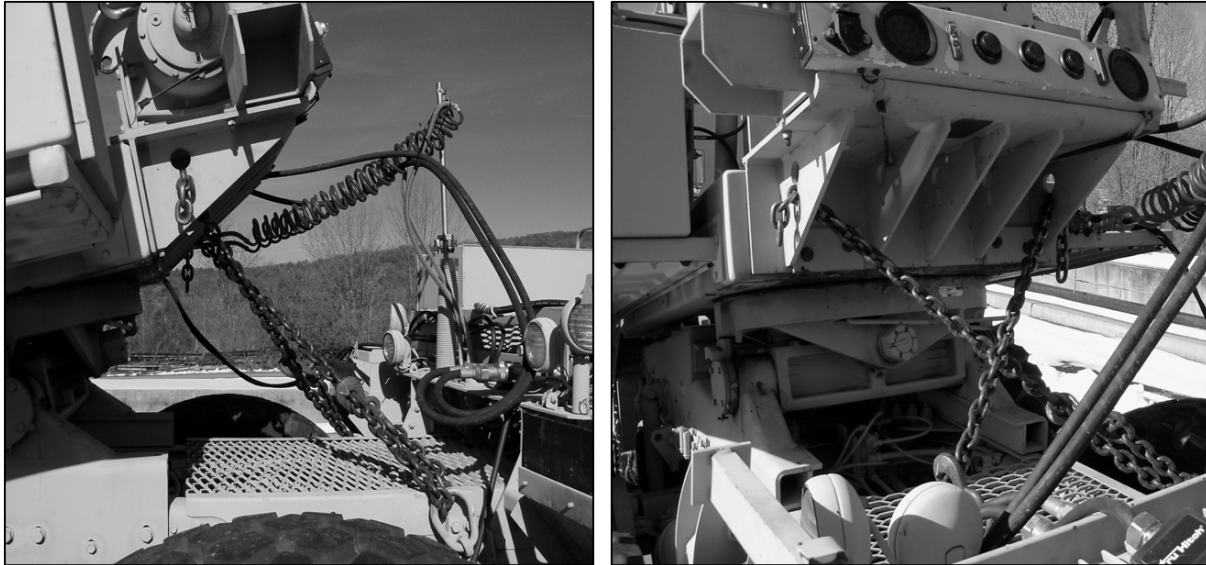
Figure 3 - Cross chain points FWTRD to prime mover
