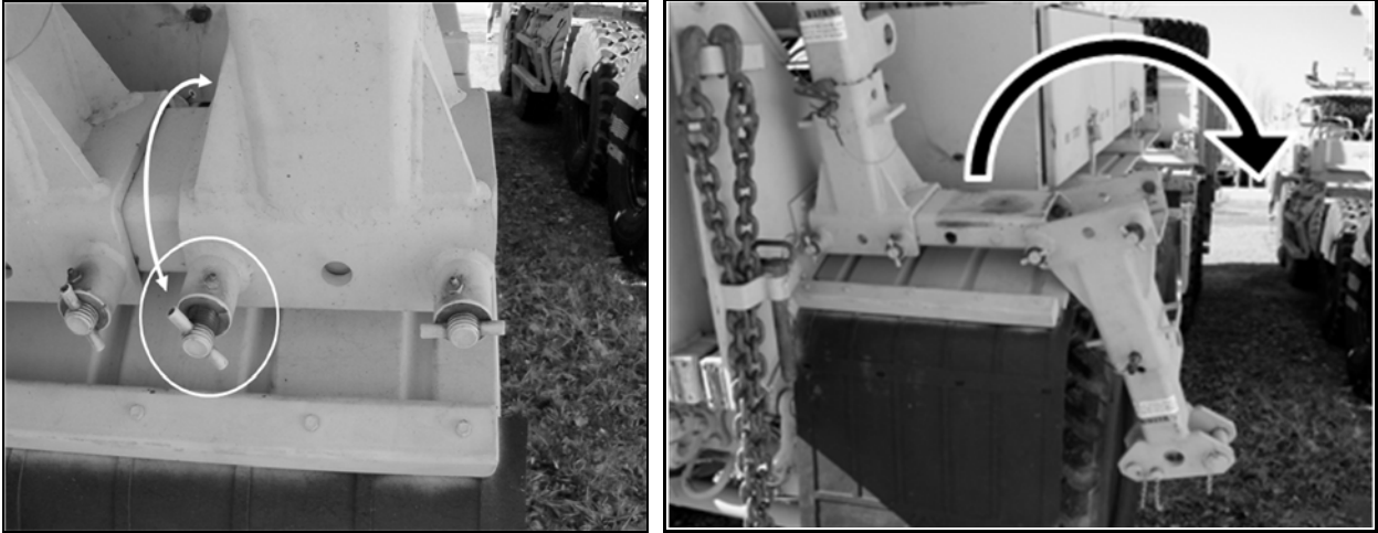
Figure 3 – Outer Tow Bar Assembly tilted away
