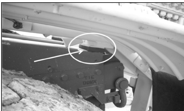
Figure 2 – Main frame support pad resting on the after frame of the prime mover. (Left side shown)
