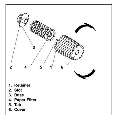
Figure 42. Type "B" Air Cleaner Assembly
