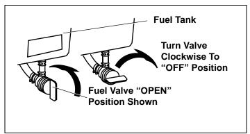
Figure 16. Optional Fuel Valve Positions
