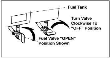
Figure 27. Optional Fuel Valve Positions
