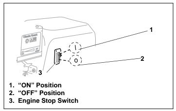
Figure 13. Engine Stop Switch
