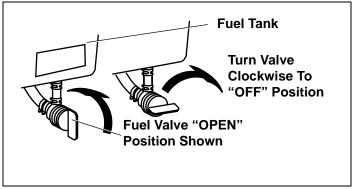
Figure 20. Optional Fuel Valve Positions
