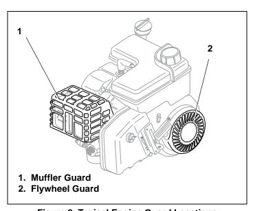
**Figure 2. Typical Engine Guard Locations**
