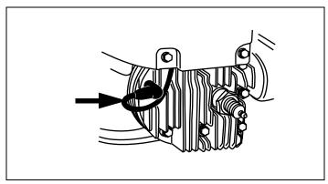
Figure 4. Spark Plug Grounding Post
