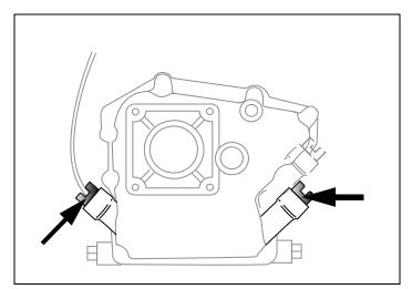
Figure 12. Possible Oil Fill Plug Location(s)
