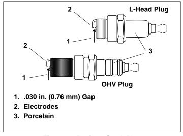
Figure 40. Resistor Spark Plug
