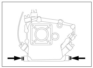
Figure 37. Possible Oil Drain Plug Location(s)
