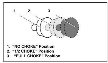
Figure 23. Remote Choke Control Positions
