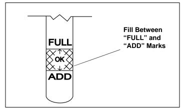
Figure 10. Engine Oil Level
