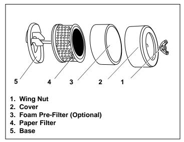
Figure 43. Type "C" Air Cleaner Assembly
