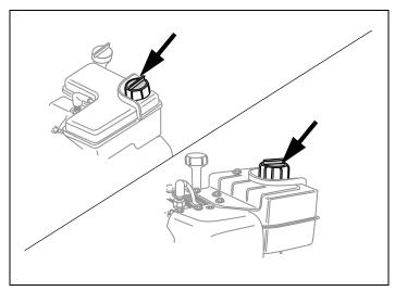
Figure 14. Possible Fuel Fill Cap Location(s)
