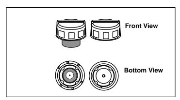
Figure 15. Possible Fuel Fill Cap(s)
