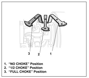
Figure 22. Horizontal Mount Choke Control Positions
