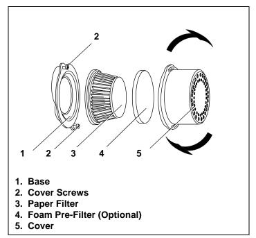
Figure 41. Type "A" Air Cleaner Assembly
