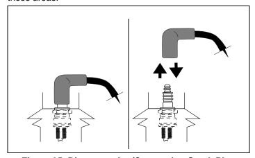
Figure 35. Disconnecting/Connecting Spark Plug
