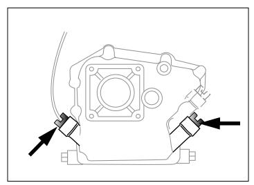
Figure 38. Possible Oil Fill Plug Location(s)
