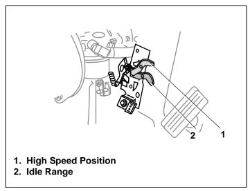
Figure 34. Engine Speed Control Positions
