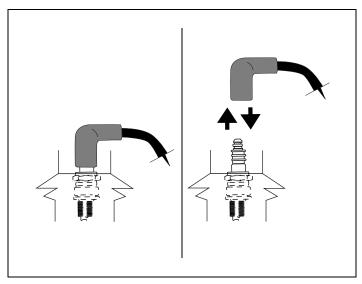
Figure 3. Disconnecting/Connecting Spark Plug
