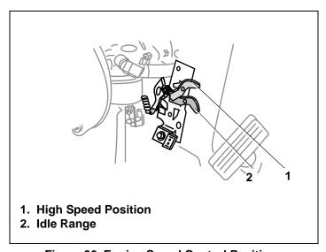
Figure 26. Engine Speed Control Positions
