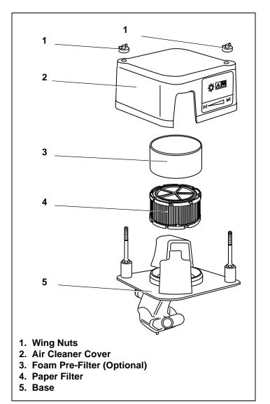
Figure 45. Type "E" Climate Guard Air Cleaner Assembly
