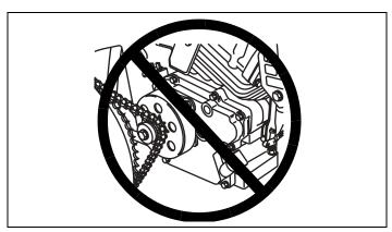
Figure 1. DO NOT use Without Engine Shaft Guard
