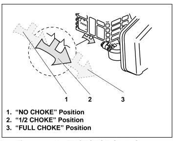
Figure 24. OH195EA/EP/XA/XP Choke Control Positions
