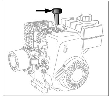
Figure 11. Possible Oil Fill Dipstick Location
