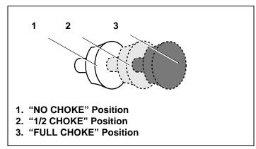
Figure 31. Remote Choke Control Positions
