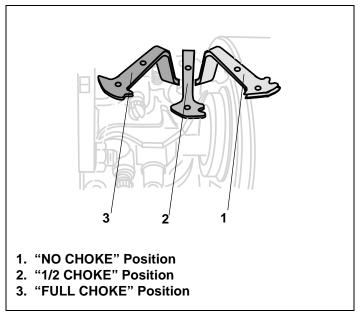
Figure 30. Horizontal Mount Choke Control Positions
