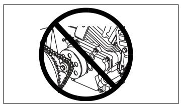
Figure 7. Incorrect Usage Without Engine Shaft Guard
