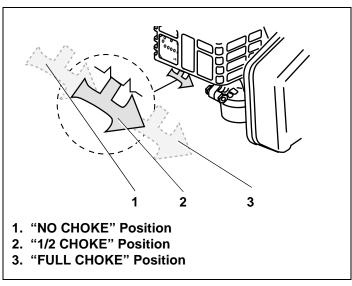
Figure 32. OH195EA/EP/XA/XP Choke Control Positions
