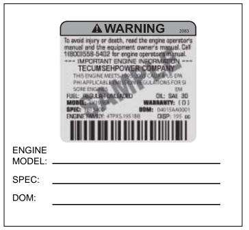
Figure 5. Engine Identification Decal
