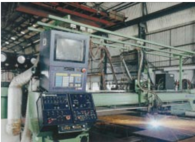
CNC Gas cutting machine for plate cutting ensures precision cutting of shell plates and profile cut tube plates.
