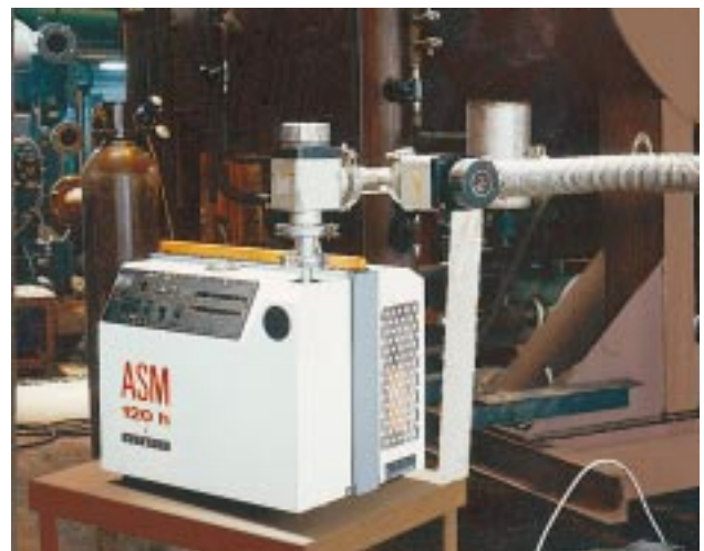
A Helium leak detection test ensures there is no leakage at the welding joints.
