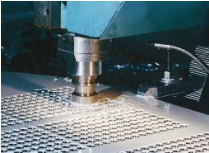
CNC drilling machine with high speed and direct feed technology ensures fine tube hole finish and accuracy, which is important for leak tight expansion and effective heat transfer.
