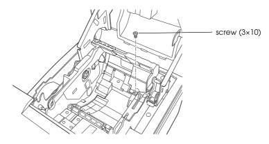
When attaching it, align the hole on the roll-paper holder for hanging bracket with the dowel on the roll paper guide.
