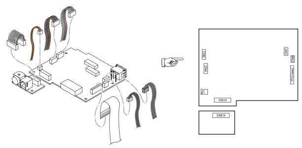
CN2: Connecting the cable of the Auto cutter unit (113)
