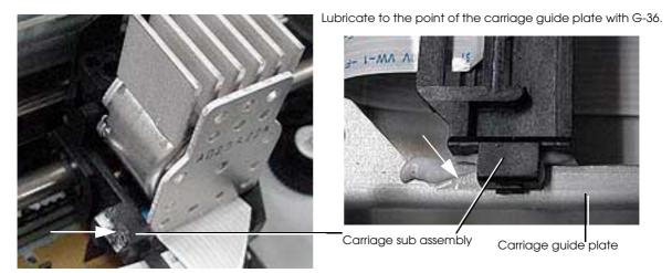
Lubricate to the switching points of the carriage guide plate sub assembly (ribbon switch lever) with G-36.
