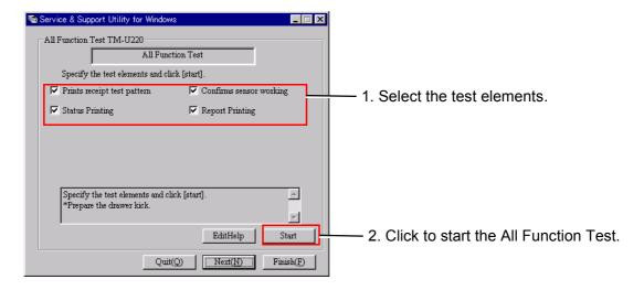
Select the test elements and click the Start button to start the all function test.
