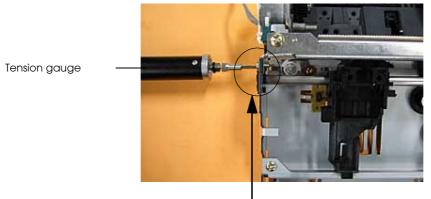
Hook the end of the tension gauge and adjust the tension
