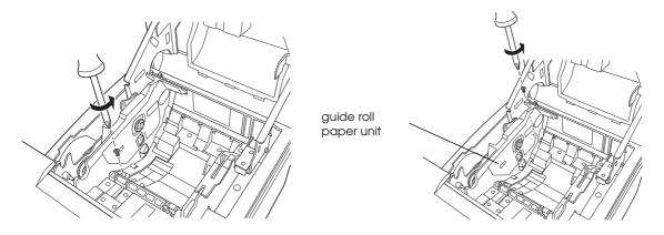
4. Rotate the detector lever on the roll paper guide to change its direction.
