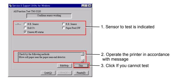
When the sensor detects the printer operation correctly, OK is displayed.
