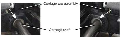
Lubricate to the point of the carriage sub assembly with G-36.
