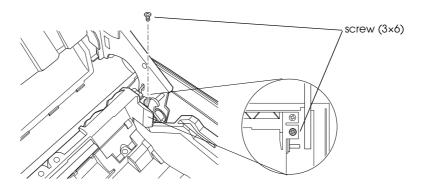
4. Remove the screw(3x6) and remove the roll paper holder for hanging bracket.
