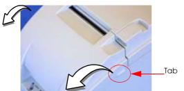
2. Open the ribbon cassette cover of the printer, using the tabs on each side of the cover.
