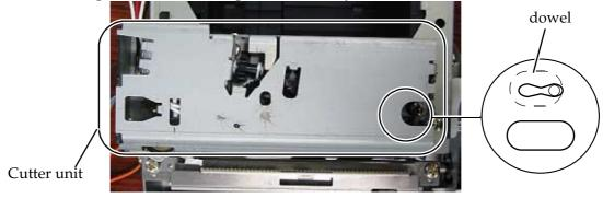
5. When you select partial cut (default), you have to adjust the dowel to the right, as shown. When you select full cut, you have to adjust the dowel to left as shown.
