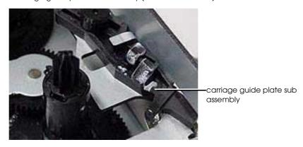
Lubricate to the point of contact between the rotation shaft and base frame (2 points) with G-36.
