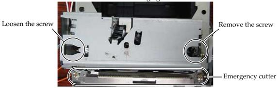
4. Lift the top of the cutter unit upward towards you and remove from the dowel.
