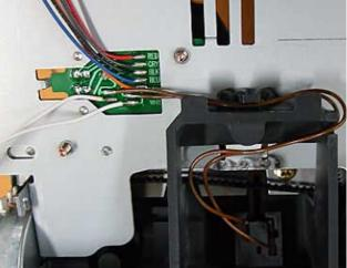
When attaching the HP board assembly, be sure that the wires is thrown to the hole, and attached the board to the
