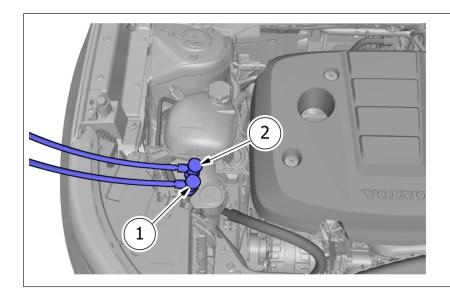
Note! When vacuum pumping, the recovery unit must be connected to both the high pressure side's (1) and low pressure side's (2) service valves at the same time.
