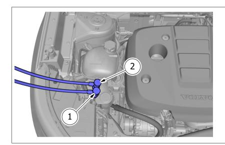
Note! When draining, the recovery unit must be connected to both the high pressure side's (1) and low pressure side's (2) service valves at the same time.
