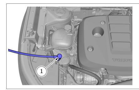
Note! Only top up refrigerant via the high pressure side's (1) service valve.
