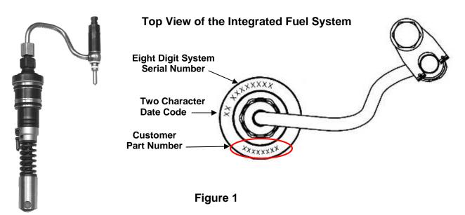
Component markings are also located on the Unit Pump Assembly, Compact Pencil Nozzle<sup>®</sup> (CPN), and the tappet assembly. These markings will be explained in detail at a later date as additional servicing of the IFS is allowed.
