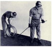
The Wrong Way To Uncoil. If a coil of wire rope is laid flat on the floor and uncoiled by pulling it straight off, spirals will occur and kinking is likely. Torsions are put into the rope by every loop that is pulled off, and the rope becomes twisted and unmanageable. Also, wire rope cannot be uncoiled like fiber rope. Pulling one end through the middle of the coil will only result in kinking.
