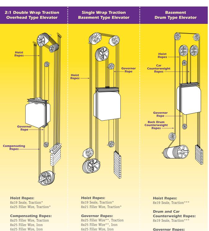
**Governor Ropes:** 8x25 Filler Wire\*\*, Traction 8x25 Filler Wire\*\*, Iron 6x25 Filler Wire, Iron
