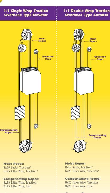
**Governor Ropes:** 8x25 Filler Wire\*\*, Traction 8x25 Filler Wire\*\*, Iron 6x25 Filler Wire, Iron **Governor Ropes:** 8x25 Filler Wire\*\*, Traction 8x25 Filler Wire\*\*, Iron 6x25 Filler Wire, Iron
