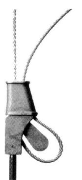
Figure 8: Seat the rope and wedge into the socket by quickly pulling the dead end
