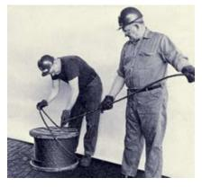
Uncoiling The Right Way To Uncoil. There is only one correct way to uncoil wire rope. One person must hold the end of the rope while a second person rolls the coil along the floor, backing away. The rope is allowed to uncoil naturally with the lay, without spiraling or twisting. Always uncoil wire rope as shown.
