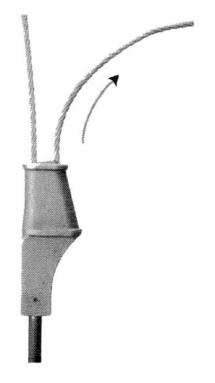
to bind the dead end to the live, or load bearing, end of the rope. Place the first clip a maximum of four times the rope's diameter above the socket, and the second clip within eight times the rope's diameter above the first clip. The purpose of the clips is to retain the wedge and prevent the rope from slipping should the load be removed for any reason.
