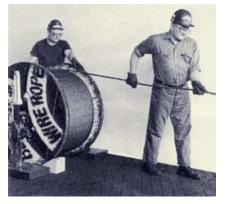
**The Wrong Way To Unreel.** If a reel of wire rope is laid on its flange with its axis vertical to the floor and the rope unreeled by throwing off the turns, spirals will occur and kinks are likely to form in the rope. Wire rope should always be handled in a way that neither twists nor unlays it. If handled in a careless manner, reverse bends and kinks can easily occur.
