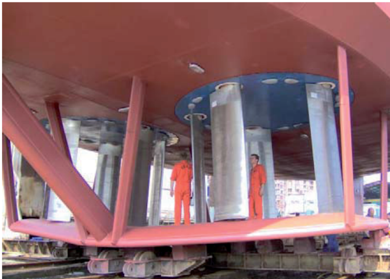
Figure 4. Voith Schneider propulsion concept with vertical axis technology [22]
