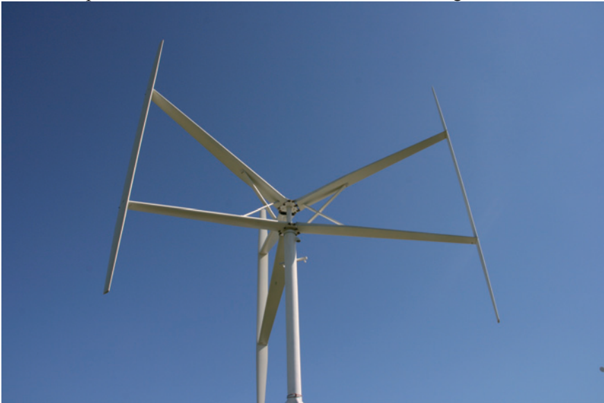
Figure 30. Marsta 12 kW turbine
