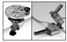
The Skiver sands the belt ends to make an overlapped joint. Once glued, the Heat Press is used for hot joining the belts after they are skived.
