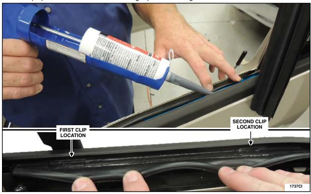
14. Using a small plastic trim removal tool, install Foam A to the outer belt moulding on top of the bead of silicone that was previously applied in Step 13. Both outer belt moulding clips need to be covered by the Foam A. See Figures 13 and 14.
