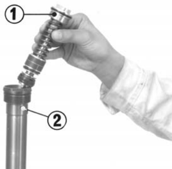
(1) FORK DAMPER (2) PISTON ROD
