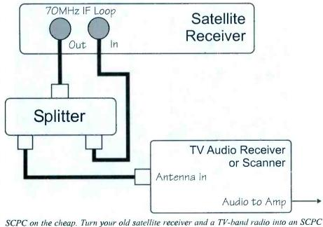
SCPC on the cheap. Turn your old satellite receiver and a TV-band radio into an SCPC receiver!
