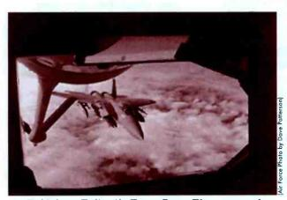
An F-15 from Eglin Air Force Base, Fla., approaches the boom of a 157th Air Refueling Wing KC-135 to receive fuel.
