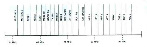
Typical (not actual) FM/SCPC single transponder service assignments on a full transponder.
