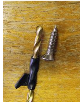
Illustration 7: Bit depth marking
