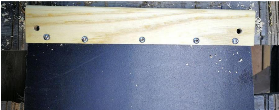
Illustration 12: Headboard layout showing location of screws and hole to accept running line.
