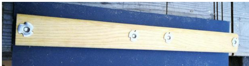
Illustration 10: Location of 4 through-bolts on tail crossbar.
