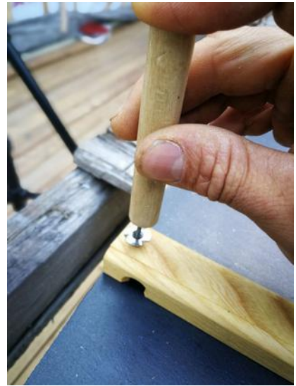
Illustration 9: Marking the bolt location in the centre of the nut.
