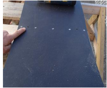
Illustration 11: Hole location in CB#2 for Haul Lines
