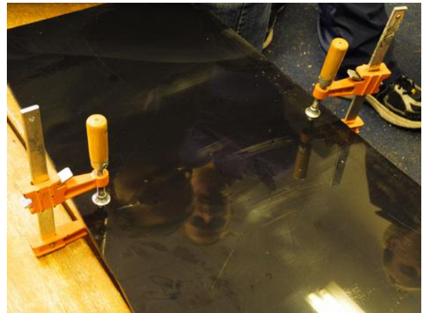
Illustration 6: Elevating the centre of the toboggan (on the 2x4) makes slipping clamps in much easier.
