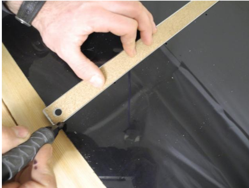
Illustration 5: Use the pre-drilled holes to place marks that will later help in aligning crossbars.
