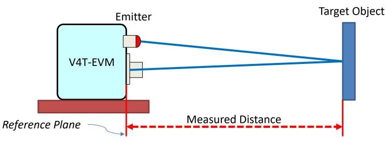
Light scattering occurs due to unwanted reflections within the optics. This cannot be eliminated completely. In order to avoid scattered light issue as much as possible, V4T-EVM should be placed at the greatest distance possible from disturbing object from which light might be reflected.
