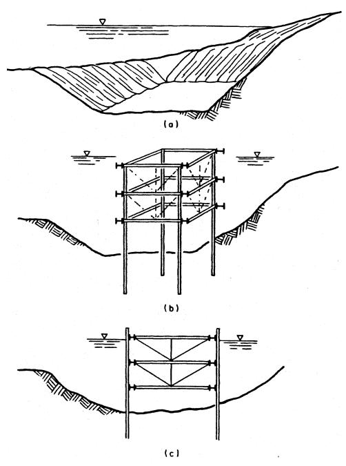
**Figure 6** – Cofferdam construction sequence (I). (a) Pre-dredge. (b) Drive support piles; set prefabricated bracing frame and hang from support piles. (c) Set sheet piles; drive sheet piles; block and tie sheet piles to top wale.
