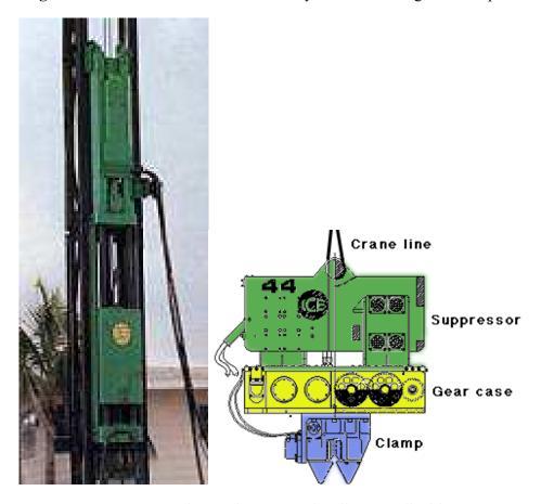
Figure 13 – An impact hammer and a vibratory pile driver
