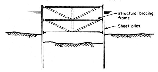
Figure 4 – Typical cofferdam without seal or pile
