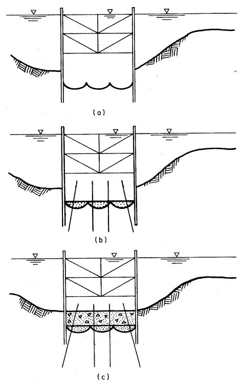
**Figure 7** – Cofferdam construction sequence (II). (a) Excavate initial and final grade. (b) Drive bearing piles in place. (c) Place tremie concrete.
