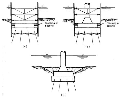
**Figure 8** – Cofferdam construction sequence (III). (a) Check blocking; dewater; construct footing block; block between footing and sheet piles. (b) Remove lower bracing; construct pier pedestal; construct pier shaft. (c) Flood cofferdam; pull sheets; remove bracing; backfill.
