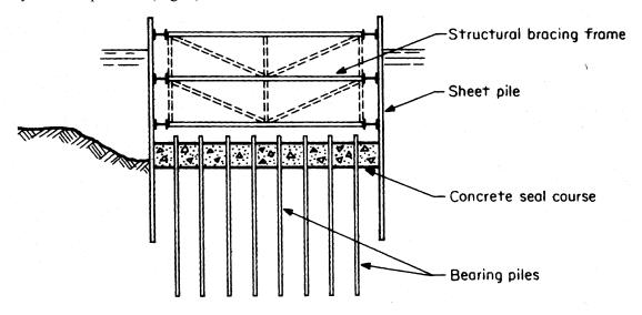
Figure 5 – Typical cofferdam (with seal)
