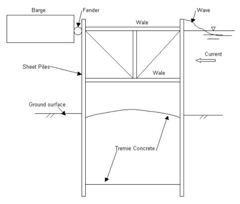
Figure 0 – Typical cofferdam schematic
