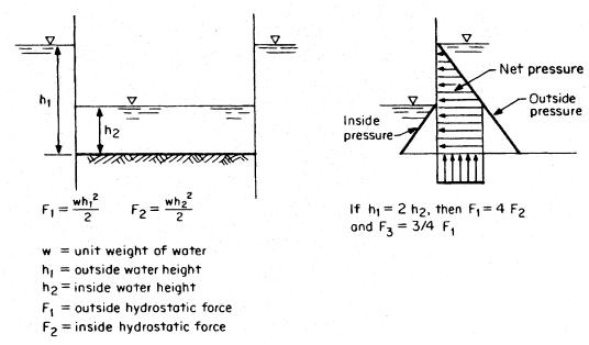
Figure 1 - Hydrostatic forces on partially dewatered cofferdam
