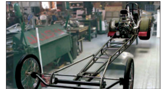
GSTAs 8th Dragster- The powerplant is an all aluminum, alcohol injected 414" Rodeck tall block
