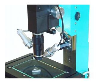
WM2 with tube **MS2-309** with a zoom objective and zoom auxiliary lens **ZV-x**
