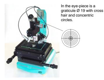
WM2 with tube **MS2-301** for inclined monocular **MS2-407**
