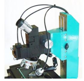
The microscope tube, consisting of components from our modular component system, can be focused on the measuring object with a coarse guiding block (dovetail guiding, rack and pinion) **B40-G** or a coarse / fine guiding block with roller guides **B40-KR**.
