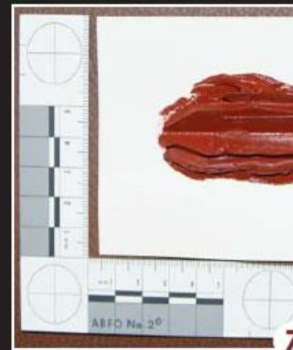
Figure 2: Photograph of the tool mark with scale. Figure 3: Misting the outlined tool mark area with silicone emulsion spray. Figure 4: Injecting polyvinylsiloxane into the tool mark. Figure 5: Fingerprint card placed over the impression material and adhered to the orthodontic wax. Figure 6: Labeled fingerprint card. Figure 7: Final impression.
