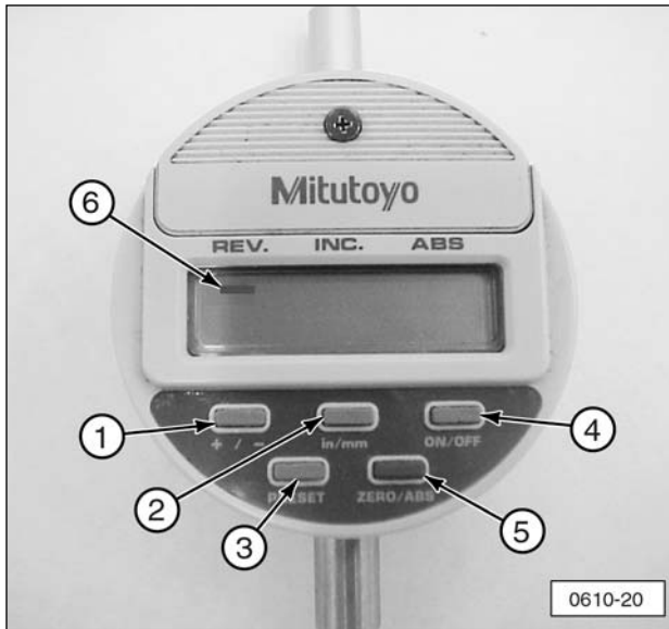
1U-8869 Digital Position Indicator (Former Style). (1) Positive/Negative Select Button. (2) Inch/ Millimeter Select Button. (3) Preset Button. (4) On/Off Button. (5) Zero/ABS Button. (6) Indicator Bar.
