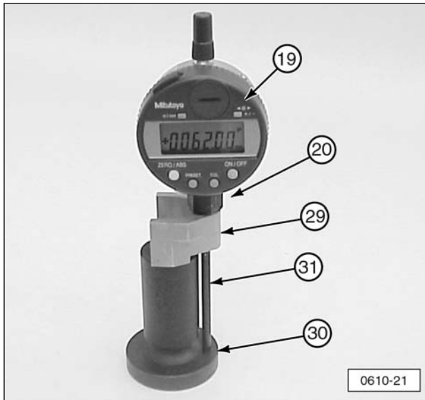
Indicator Group (Current Style). (19) 1U-8869 Digital Position Indicator. (20) 9U-6272 Nylon Holding Screw (Part Of 9U-7282). (29) 123-4940 Indicator Fixture Group. (30) 9U-7269 Timing Gauge Block. (31) 9U-7274 Contact Point.
