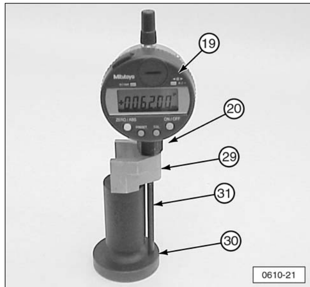
Indicator Group (Current Style). (19) 1U-8869 Digital Position Indicator. (20) 9U-6272 Nylon Holding Screw (Part Of 9U-7282). (29) 123-4940 Indicator Fixture Group. (30) 9U-7269 Timing Gauge Block. (31) 9U-7274 Contact Point.
