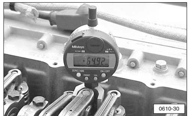
Timing Fixture Installed (Current Style).
