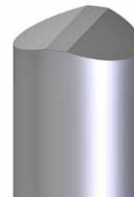
Figure 3-20. A chamfered punch with a flat centre section.
