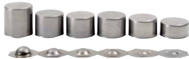
Figure 3-3. Maximum- cup height and dome height for deep drawing and stretch forming, respectively. Steel grades (from left to right): DC06, Docol 600 DP, Docol 800 DP, Docol 1000 DP, Docol 1200 M and Docol 1400 M.
