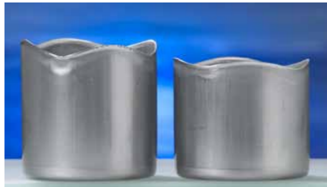
Figure 4-1. The influence of lubricant viscosity on drawing. Maximum cup height using lubricant viscosity 500 cSt (left cup) and 40 cSt (right cup).
