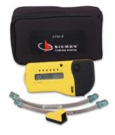
STM-8-S ...... Shielded twisted-pair tester. Includes carrying case,
