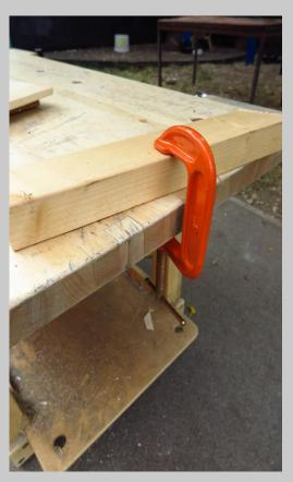
HOLD WORK STEADY WITH A G-CLAMP- ESPECIALLY USEFUL FOR DRILLING
