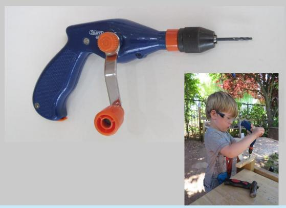
MAKE LIFE EASY WITH A HAND DRILL- MAKING PILOT HOLES FOR SCREWING AND HOLES TO MAKE JOINING WITH NAILS EASIER
