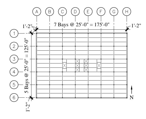
Example 7-story **Building: Shallow foundations** designed for perimeter frame and core bracing.
