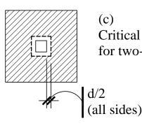
(c) Critical section for two-way shear
