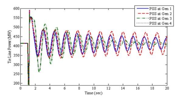
Figure 7: The tie line power of the system with a single PSS installed
