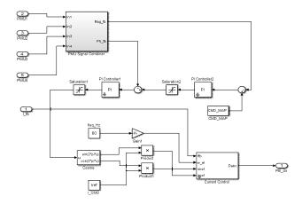
Figure 14: RFLC load controller architecture
