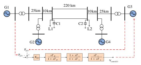
Figure 8: Test system with the remote feedback controller
