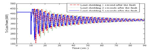
Figure 12: Tie Line power with load shedding with different delays
