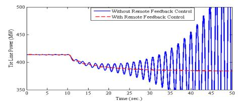
Figure 9: The tie Line power of the system without a controller vs remote feedback control at Gen 3 Comparison between single PSS system and RFC retrieves faster oscillation damping, Figure 10.
