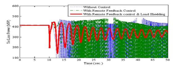
Figure 11: Line trip after 10 seconds with and without load shedding
