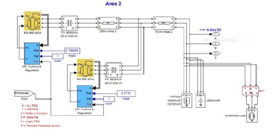
Figure 5: Area 2 subsystem with switchable loads
