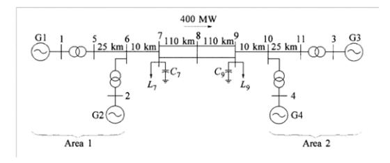
Figure 3: Test System, extracted from [12]
