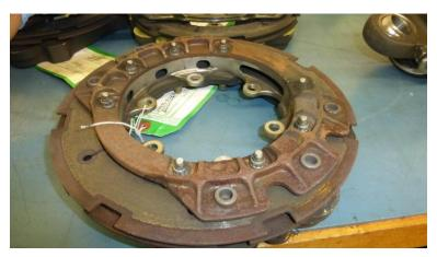
Main Landing Gear Brake Assembly
