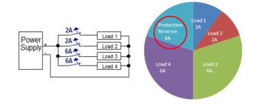
With an Electro-Mechanical circuit protection device (a fuse or MCB) the circuit designer must account for additional current that may be required to trip the fuse or circuit breaker (Reserve for Protection).
