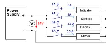
The 1 A loads typically are fused at 2 A and the 3.5 A loads are fused at 6 A. The tripping current for a fuse is about 1.8 times the fuse value so the current required to trip the fuse is shown in the table below:
