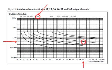
Using Bulletin 1692 ECP, this fault current on a 6 A circuit would be sensed about 300 ms.
