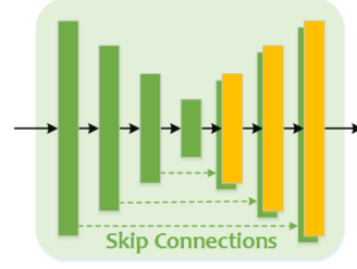
Fig. 4. Architecture of the U-Net. The skip connections between networks are illustrated as dotted arrows.
