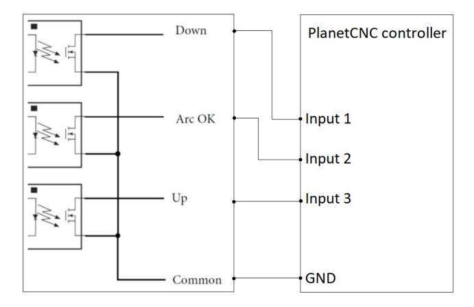
Please note that Down, Up, Arc OK signals can be connected to any input of PlanetCNC controller since inputs function can be configured later in PlanetCNC TNG settings.
