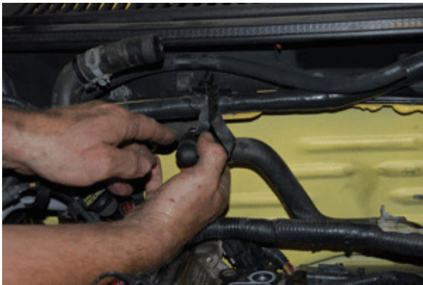
Disconnect water heater hose (rear on manifold to firewall) from firewall. (snap connector)
