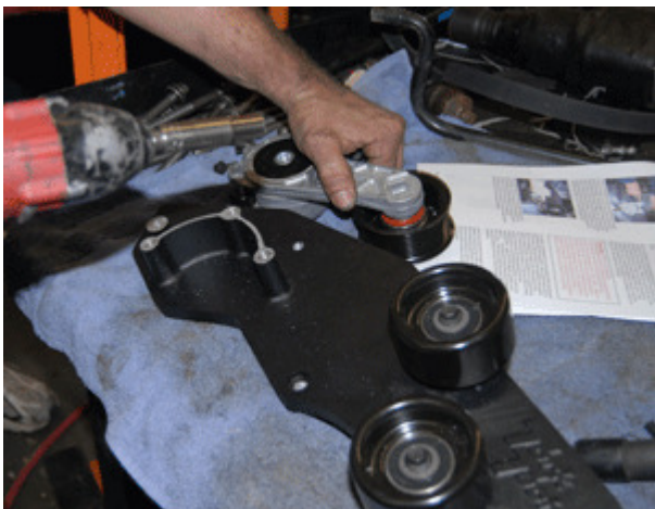
A new tension arm that is included in our kit will likely be attached to the cross brace assembly but take out the 3 bolts and remove it before attaching the cross brace to the two studs.
