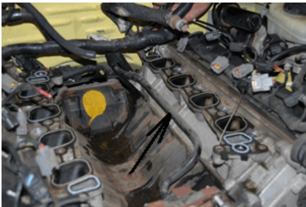
Disconnect water heater hose (rear on manifold to firewall) from firewall. (snap connector)
