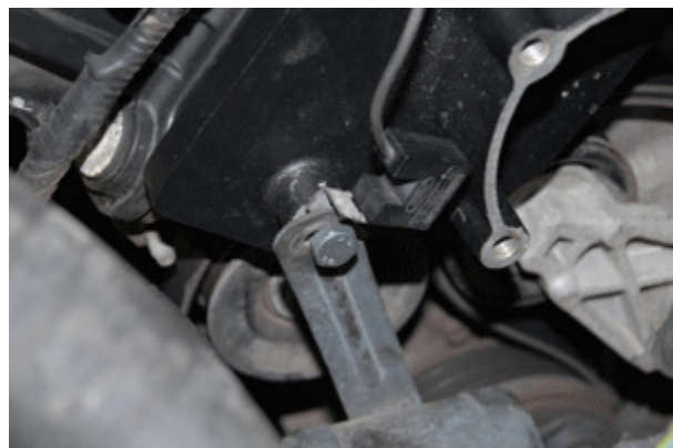
Refasten the 3 bolts that hold the new tension arm to the cross brace.
