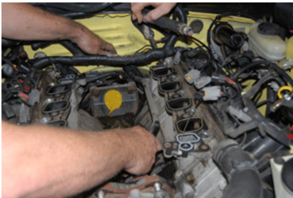
Remove the remainder of this coolant line (see arrow) that goes from the firewall to the front of the valley of the block. Also unclip the 90 degree fitting that feeds this coolant line into the heater core on the firewall.
