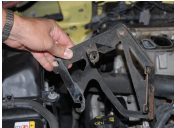
Remove the power steering reservoir and its mounting bracket.
