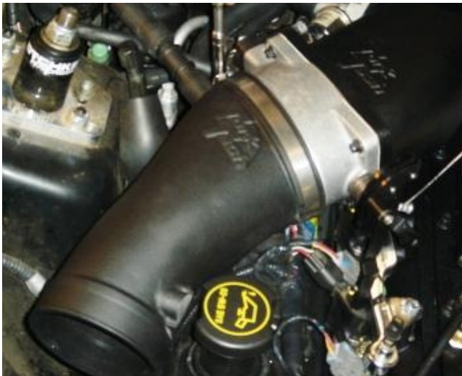
Shown above is the optional TTI intake tube between the MAFS and Tbody for reference.
