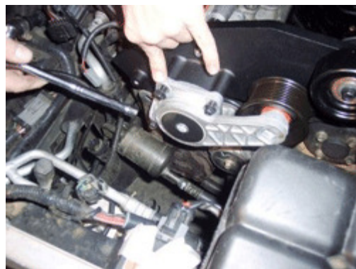
Refasten the 3 bolts that hold the new tension arm to the cross brace.
