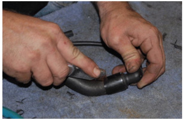
Use a knife to cut off the reinforcement wrap near the 90 degree fitting and also remove the line from the fitting as we will be reusing this fitting later. Once the fitting is separated from line you can clip it back into place on the firewall pointing towards the center of the car. A new hose will be attached to it shortly.
