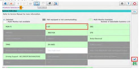
4. Wait for the **Waiting for Trigger** bar to turn green, then drive the vehicle. When you feel the vibration/shudder, hit select the Trigger icon.
