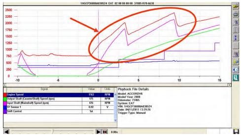
If you are dealing with a vibration caused by a faulty torque converter, you will see oscillations in the Input and Output shaft when the engine speed is smooth as shown below:
