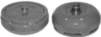
Toyota A30 - 3 Speed. With dowel pin in mounting ring.
