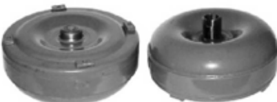
Same as R-19 with Lockup clutch omitted.
