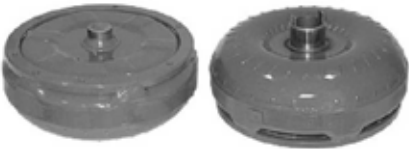
Toyota A20 - 2 Speed. With dowel pin in mounting ring.
