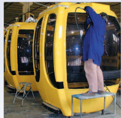
Dow Automotive BETA-MATE glass bonding systems help seal stationary glass, adding to the vehicle's structural strength and protecting the interior cabin from dirt and other environmental elements.
