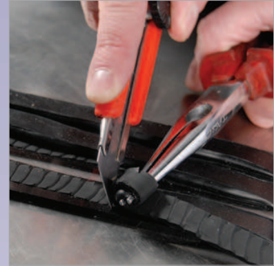
Peel strength tests enable Dow Automotive experts to quantitatively compare cut bead performance.
