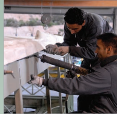
BETAMATE structural adhesives reduce vibration by stiffening overall vehicle structure.
