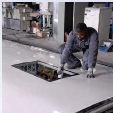
BETA-PRIME™ primer is applied to the roof surface prior to the application of BETA-MATE™ structural adhesive.
