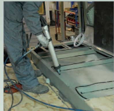
Acoustics are also improved by the use of BETAMATE structural adhesives in applications like the roof bonding (above) and the floor bonding (shown here).
