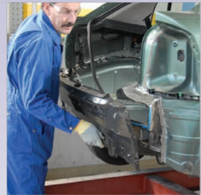
Dow Automotive structural adhesives can be used for aftermarket body repair on a variety of substrates.
