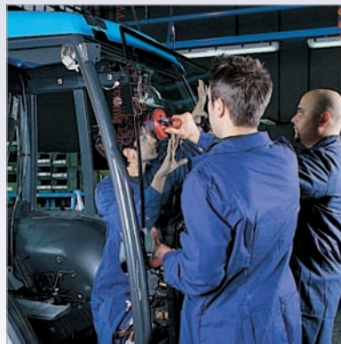
Glass bonding systems from Dow Automotive enable repaired windscreens to support a vehicle's structural integrity and return it to original manufacturer specifications.
