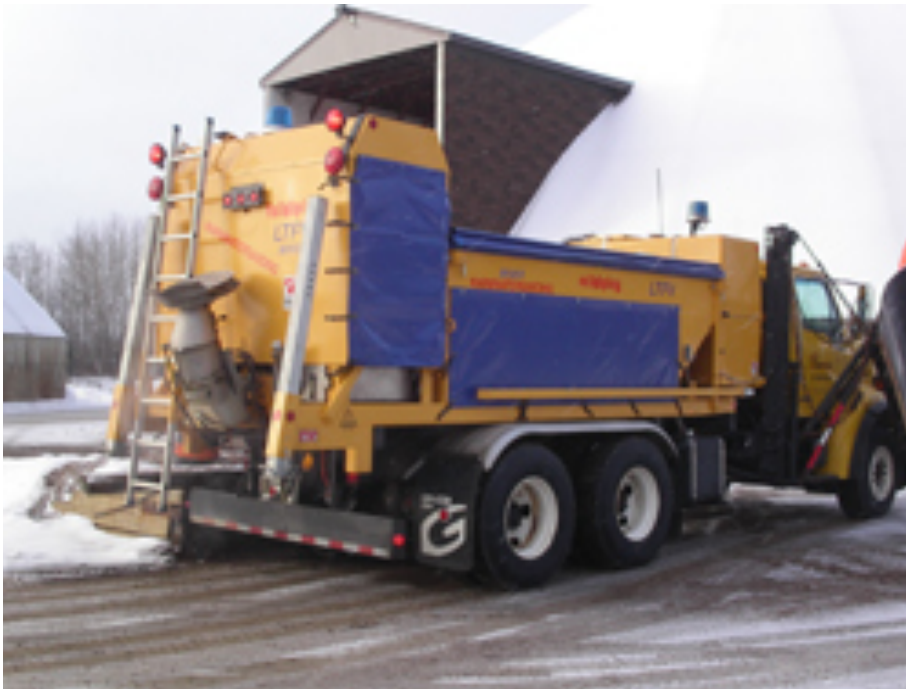
Figure 39: Falköping’s hot water/sand spreader for extremely cold temperatures.
