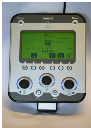
Figure 1: AEBI Schimdt's "Thermologic" controller, an example of one of the more advanced controllers.
