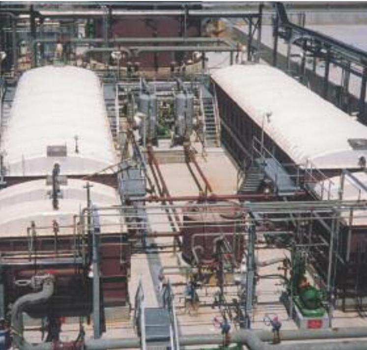
DGF separators can be completely shop fabricated with VOC containment covers. Ancillary sludge handling, activated carbon and recirculation equipment can also be provided.
