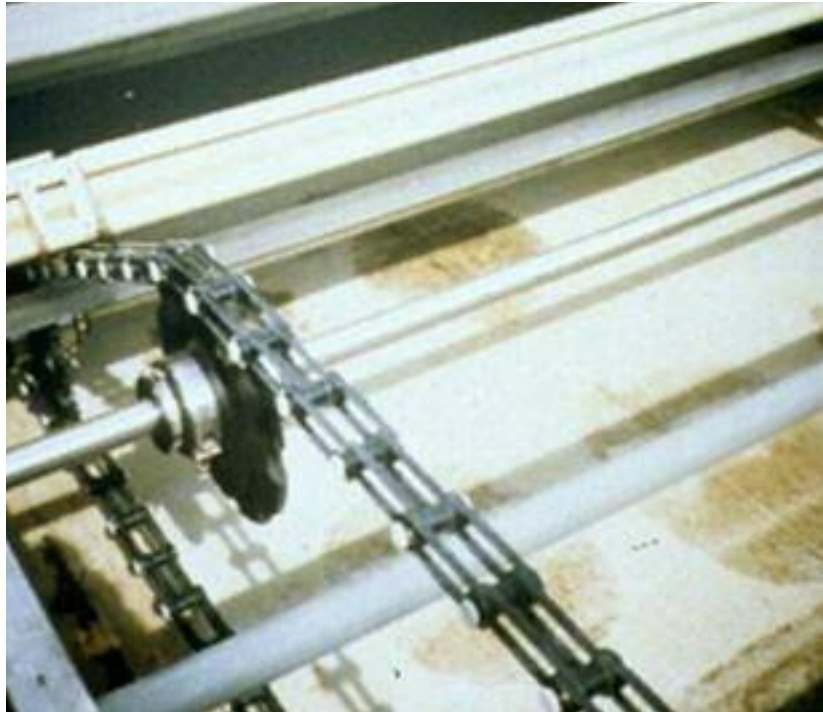
Specially designed, high-strength, light-weight, non-metallic collector components are designed to work in the high temperature and corrosive environments of the petroleum industry.
