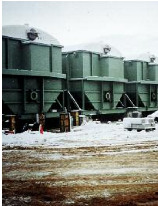
The modular design of the RBC system allows units and tankage to be completely shop fabricated.
