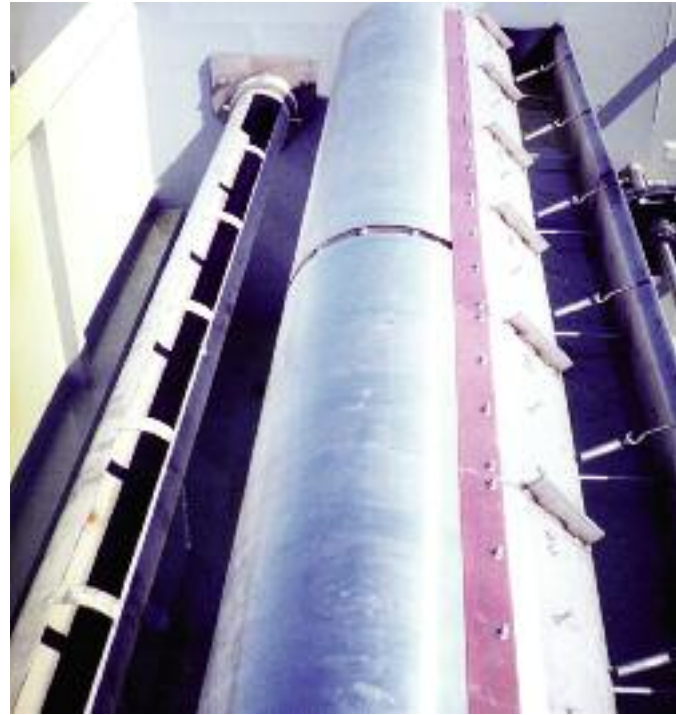
Oil roll skimmers recover up to 99 percent pure oil from API and CPI separators.
