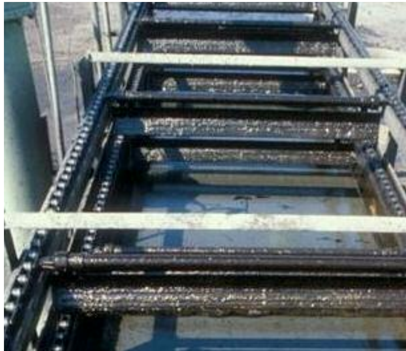
The DGF separator process combines chemical pretreatment and flotation to effectively treat and remove free and emulsified oil from desalter brine water.
