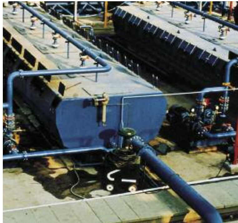
Siemens Water Technologies offers induced air flotation (IAF) and induced gas flotation (IGF) separators suited for those applications with limited space for equipment.
