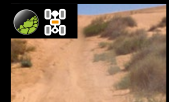
4LLC (4WD Low Range with locked centre differential) For steep hills, sand, deep snow, etc. ^
