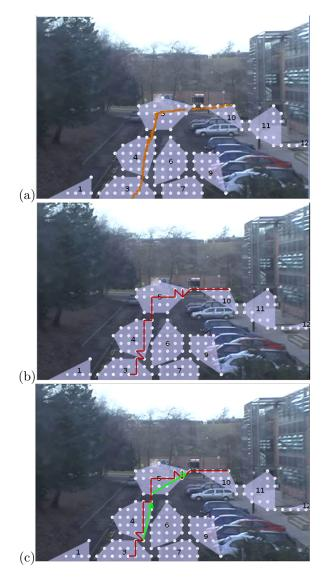
Fig. 4. Example of (a) Single Trajectory passing the zones (orange line), (b) Snapped Trajectory (red line), (c) Example of direction computation for the Snapped Trajectory in zones 4 and 5 (green arrows).
