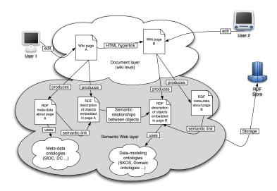
Fig. 2. Architecture of one wiki from the wiki-farm
