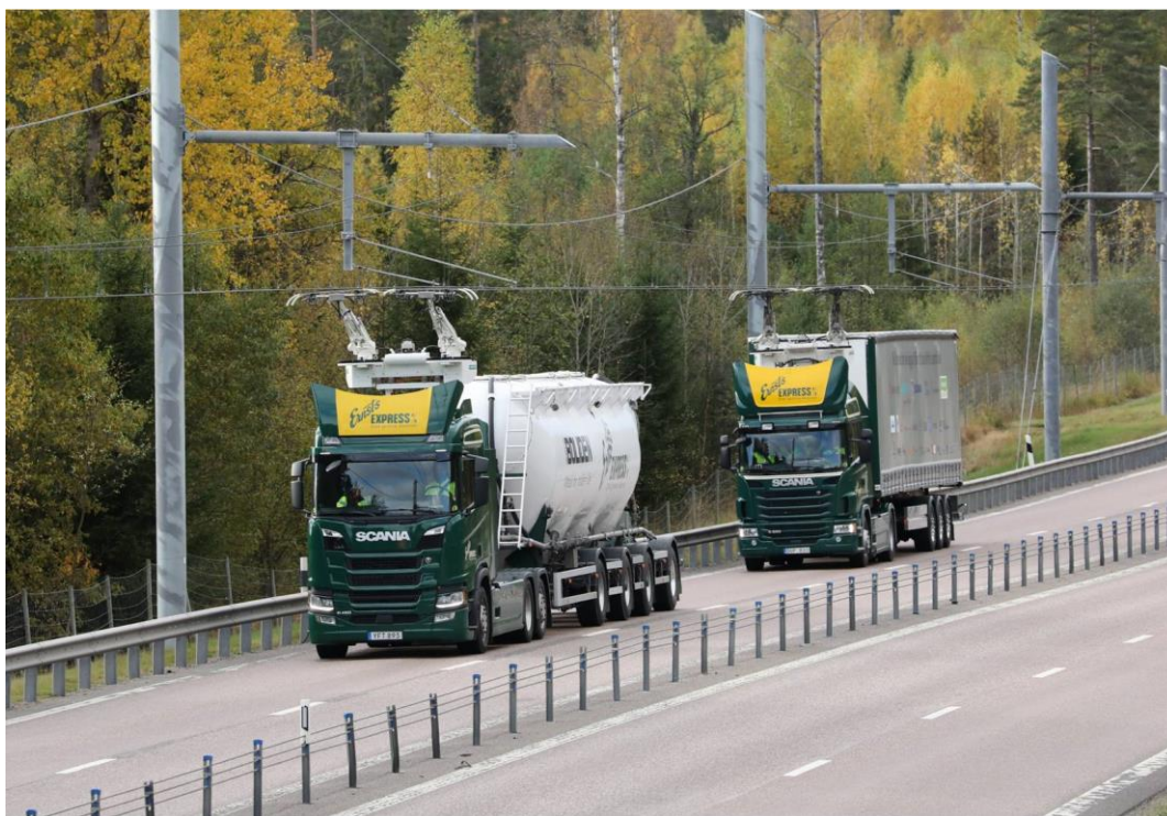
Figure 34. eHighway demonstration in Sweden
