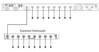
Fig 3 - Up to 16 equal level RF Outputs
