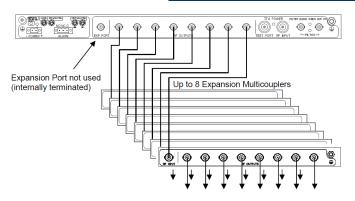
Fig 4 - Up to 64 equal level RF Outputs
