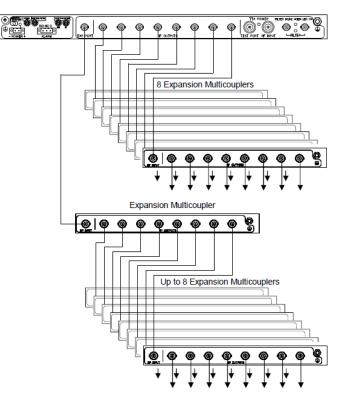
Fig 5 - Up to 128 equal level RF Outputs
