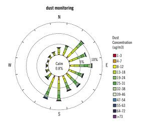
This wind rose illustrates the direction from which dust originated and the concentration of dust levels at the port. The dust monitoring unit is located on the sea end of berth 10 with the majority of port operations to the east of the unit. The wind rose illustrates that the majority of data was collected from an easterly direction
