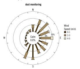
This wind rose plots wind speed and wind direction. Wind data is used to determine whether high dust levels are a result of high wind speeds or whether they are source-based. During 2001/02 higher wind speeds were recorded from an easterly and north-easterly direction. When compared with the previous graph, it can be roughly concluded that higher wind speeds were not responsible for higher dust levels. Further data analysis is required before this conclusion can be confirmed.
