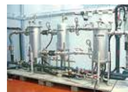
Cooling and circulating water purification systems for moulds and cooling towers
