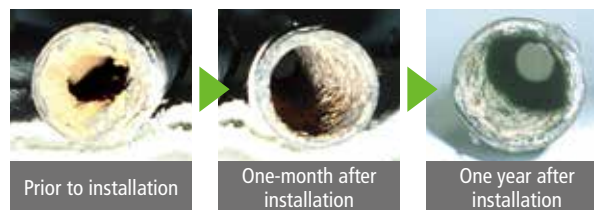
Cooling and circulating water purification systems for moulds and cooling towers
