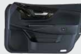
Door trim of the new model Crown that utilises high impact-resistant plastic
