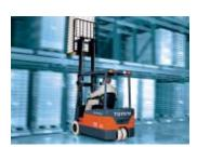
**7FBEF18**Three-Wheel Electric Counterbalanced Forklift Truck
