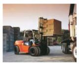
**7FGU70**Internal Combustion Pneumatic Tire Counterbalanced Forklift Truck
