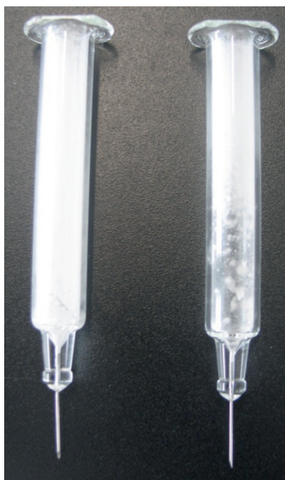
Fig. 8: Glass dust test: left – syringe siliconized with an diving nozzle, right – syringe siliconized with a fixed nozzle.
